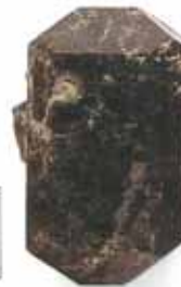
Tetragonal system represented by idocrase. Essential symmetry element: one fourfold axis.
