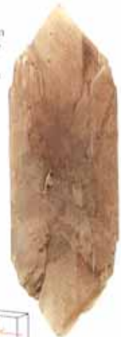
Orthorhombic system represented by barite. Essential symmetry element: three twofold axes.
