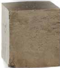
CUBE A form of six square faces that make 90° angles with each other. Each face intersects one of the fourfold axes and is parallel to the other two.
