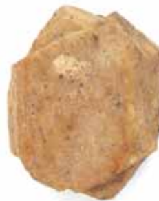
Tetragonal system represented by idocrase. Essential symmetry element: one fourfold axis.
