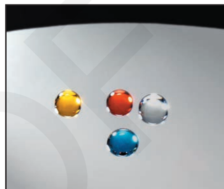
Water droplets on a (heptadecafluoro-1,1,2,2-tetrahydrodecyl)trimethoxysilane-treated silicon wafer exhibit high contact angles, indicative of the low surface energy. Surfaces are both hydrophobic and resist wetting by hydrocarbon oils. (water droplets contain dye for photographic purposes).
