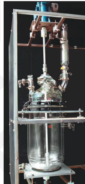
Fig. 1 Reactor for slurry treatment of powders. Separate filtration and drying steps are required.
