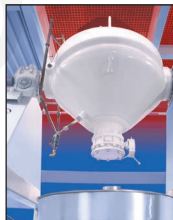
Fig. 2 Vacuum tumble dryers can be used for slurry treatment of powders.
